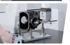
Our measuring and testing laboratory is DIN EN ISO 17025 certified. With state-of-the-art precision measuring machines 3D measurements for quality assurance and the digitisation of mouldings for reverse engineering are possible.
